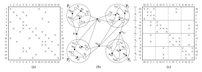
Figure 4: (a) A  $16 \times 16$  structurally nonsymmetric matrix **A**. (b) Column-net representation  $\mathcal{H}_{\mathcal{R}}$  of matrix **A** and 4-way partitioning  $\Pi$  of  $\mathcal{H}_{\mathcal{R}}$ . (c) 4-way rowwise decomposition of matrix  $\mathbf{A}^{\Pi}$  obtained by permuting **A** according to the symmetric partitioning induced by  $\Pi$ .
