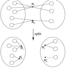
Figure 5: Cut-net splitting during recursive bisection.
