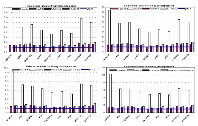
Figure 8: Relative run-time performance of the proposed column-net hypergraph model (Clique-net, hMeTiS, PaToH-HCM and PaToH-HCC) to the graph model (pMeTiS) in rowwise decomposition of symmetric test matrices. Bars above 1.0 indicate that the hypergraph model leads to slower decomposition time than the graph model.
