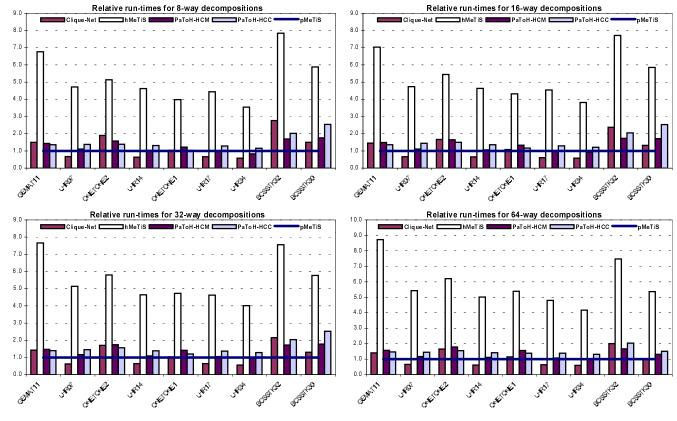
Figure 9: Relative run-time performance of the proposed row-net hypergraph model (Clique-net, hMeTiS, PaToH-HCM and PaToH-HCC) to the graph model (pMeTiS) in columnwise decomposition of symmetric test matrices. Bars above 1.0 indicate that the hypergraph model leads to slower decomposition time than the graph model.
