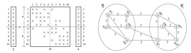
Figure 1: Two-way rowwise decomposition of a sample structurally symmetric matrix **A** and the corresponding bipartitioning of its associated graph  $\mathcal{G}_A$ .
