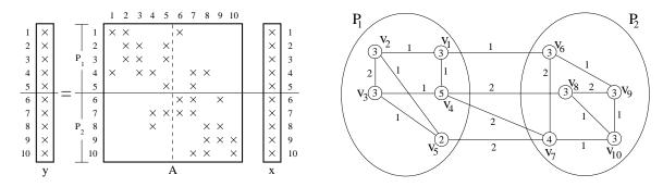
Figure 2: Two-way rowwise decomposition of a sample structurally nonsymmetric matrix **A** and the corresponding bipartitioning of its associated graph  $\mathcal{G}_{\mathcal{R}}$ .
