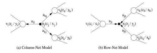
Figure 3: Dependency relation views of (a) column-net and (b) row-net models.
